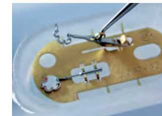
Thermo-Dummy: With a fine instrument (hook) the Thermo-Dummy is lifted out of its anchorage and moved into a vertical position.
